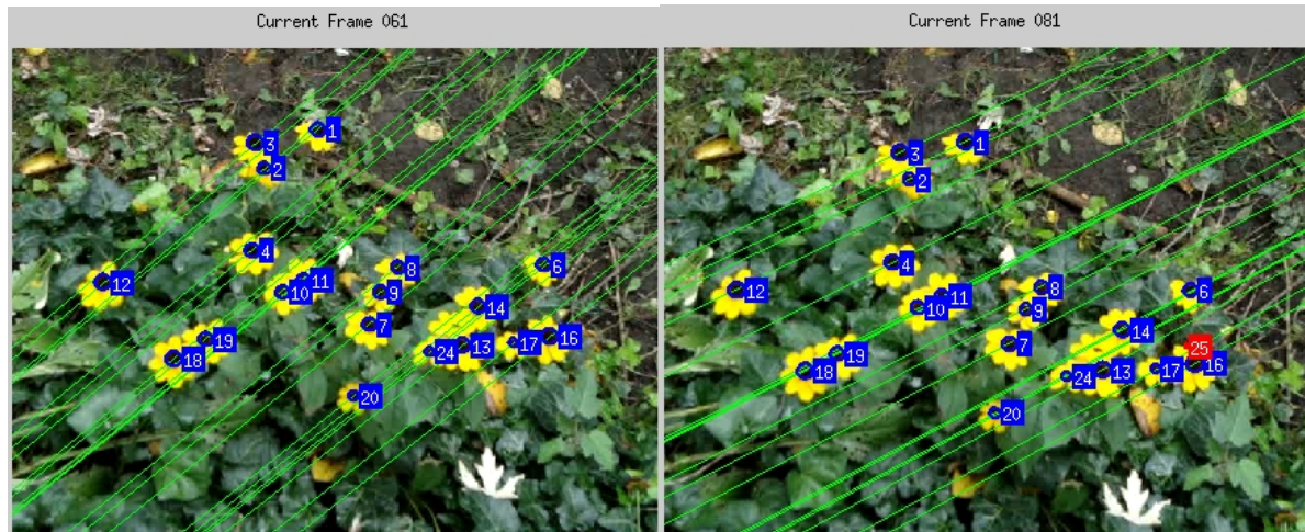
figure 8: two successive frames with labeled flowers, using homographies and iterative matching. As can be seen, all flowers are matched correctly after the last iteration of matching. The first iteration of matching would essentially be used to inform the homography, and any successive ones will refine it and produce a better matching.
