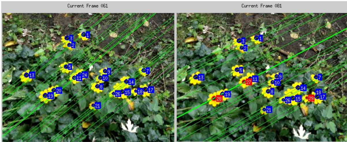
figure 7: two successive frames with labeled flowers, without using homographies and iterative matching. Flowers labeled blue in the frame on the right denote flowers that got matched to the ones from the previous frame, while those labeled red were unmatched. As you can see, the flowers labeled 20 and 24 in frame 61, were mislabeled as 19 and 11 in frame 81 respectively. This is because all 4 flowers lay on the same line, and taking the euclidian distance between the two frames without a homography resulted in a mismatch. Due to the wrong labeling of these two flowers, new labels were introduced for the flowers that should have been matched.
