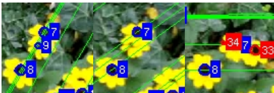
figure 13: Three frames are shown around the location of the same flowers: frames 141, 151, and 261 respectively. Flower 9 gets occluded by 7 and then emerges on the other side. Our algorithm mislabels this flower as a new one, since its movement does not follow the approximate homography of all other flowers. When it reappears in frame 261 it is treated as a new flower.
