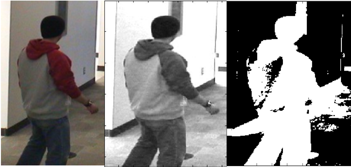
Figure 4: From left to right, the original image, its grey scale, and the segmentation result using the previously discussed optimal values of k and the number of histogram bins.
